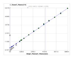
The slope K and the intercept V must be interpreted according to the underlying compartment model. For the FDG tracer, the slope K equals  $K_1k_3/(k_2+k_3)$  and represents the metabolic flux, while the intercept V equals  $V_0+vB$  with the distribution volume  $V_0$  of the reversible compartment  $C_1$  and the fractional blood volume vB.
